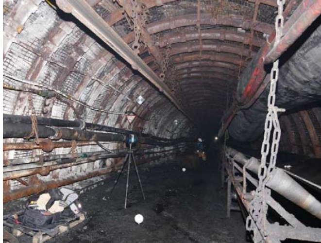
Figure 2: Scanning of the longwall roadway by Faro Focus S 350 scanner
