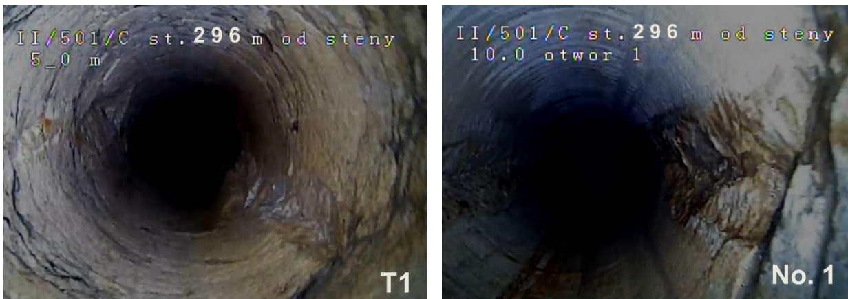
Figure 12: Example of breakouts at the exploratory borehole T1 and installation borehole No. 1
